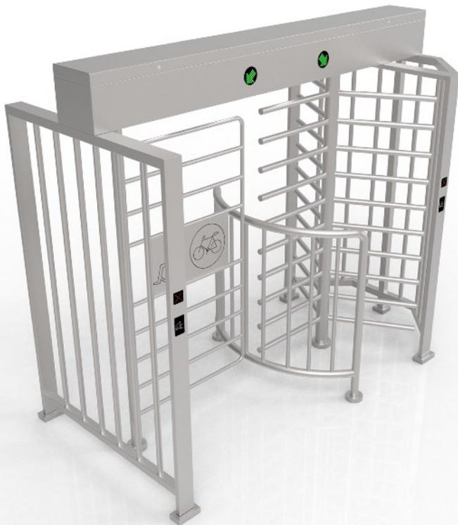
**CP451-C handicap full high turnstile** is a combine of rotor and swing gate. The rotor gate is for normal people access control and the swing handicap turnstile gate with greater clearance can be used for luggage or handicapped access. The two gates are independent from each other. Two gates can work at the same time. The gate can be free egress in case of emergencies. Further, full height turnstiles can be fitted with turnstile safety sleeves for ease of use, protection, and insulation.
