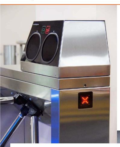
An automatic hand disinfection sprays a sanitizer when a person places their hands in the disinfection unit. In the lower part of the turnstile body there is a 5 liter tank with sanitizer liquid. The sanitizer liquid is extracted from the reservoir by vacuum pumps and sprayed onto the hand from several points. The disinfecting unit is made of stainless steel.
